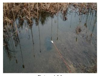
Photograph 2 🛧 Trap was tethered to trees with rope and completely submerged, resting on the pond substrate.
